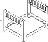
Slide the preassembled sides in the grooves of the legs to complete the sides.
