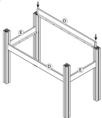
3 Slide dovetailed boards (F/G) into legs as shown.
