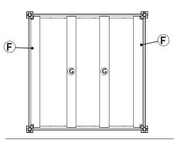
Place remaining bottoms boards (G) on the four bracing boards, perpendicular to the bracing boards. Note: Boards will have small gaps in between them to allow for drainage.
